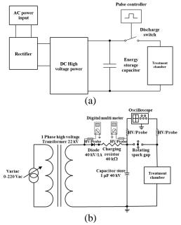
**Fig. 1.** The designed PEF system: (a) PEF operation, (b) schematic diagram.
