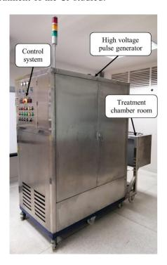
**Fig. 4.** The PEF system for CJ treatment.
