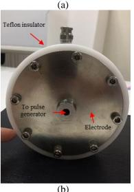
**Fig. 2.** Treatment chamber for the study: (a) schematic diagram of chamber, (b) photograph of treatment chamber.
